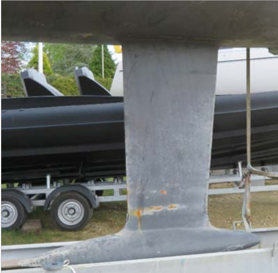
Figure 6: Comar Comet 45S, deep draught racing keel (not fitted to Tyger of London )
