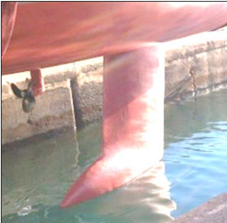
Figure 7: Comar Comet 45S, shallow draught, lead, cruising keel fitted to Tyger of London
