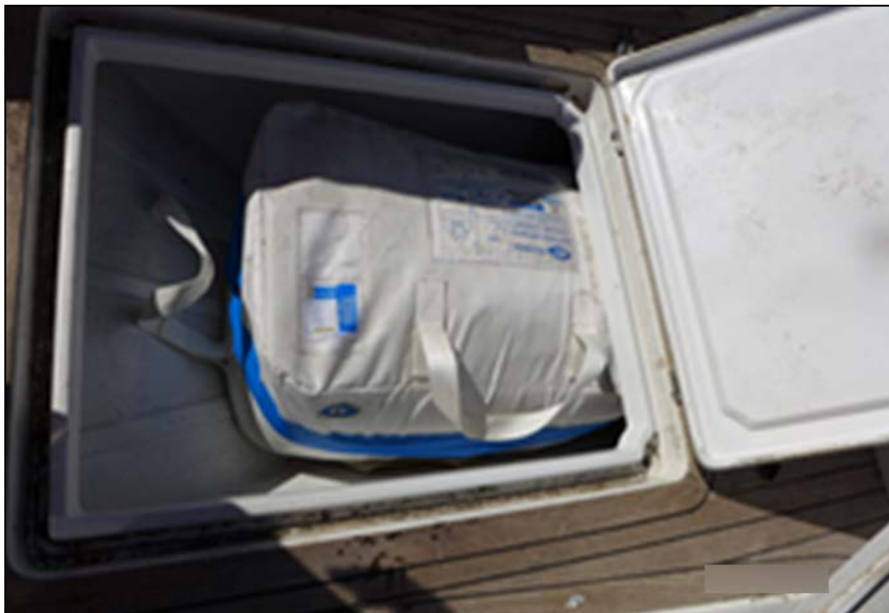
Figure 12: Tyger of London's valise liferaft, post-accident, in its cockpit locker
