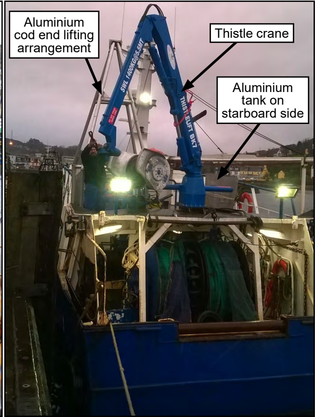
Figure 5b: Nancy Glen – replacement Thistle crane
