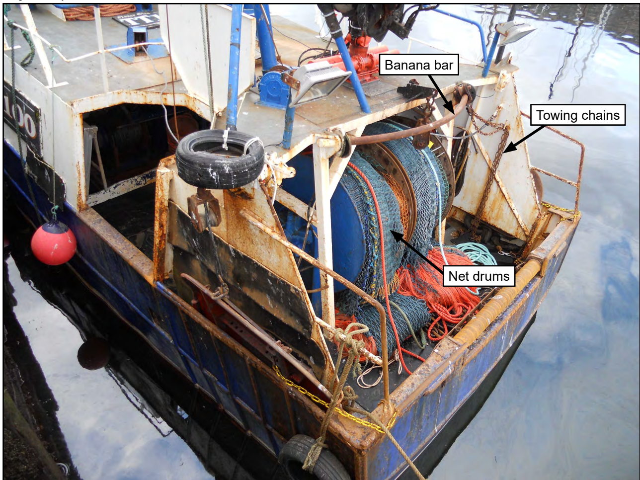
Figure 7: Nancy Glen's trawling arrangement showing the net drums, towing chains and banana bar
