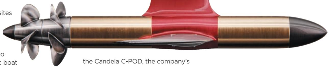
the Candela C-POD, the company’s proprietary electric drive train. Next in the pipeline is a 40ft foiling passenger ferry in Stockholm and the company says it plans to rapidly expand its model programme, with a larger leisure boat following on from the R&D gathered.
